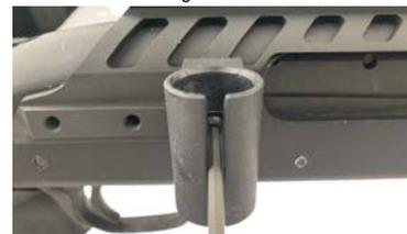
Place the add-a-shell onto the side saddle and using the provided 10-32 x 3/8" button head screw (#1) and the lock washer (#4), tighten the add-a-shell to the side saddle using a 1/8" allen wrench as seen in (Figure 2a). You may mount up to 6 add-a-shells to the non-ejection port side and up to 3 on the ejection port side.
