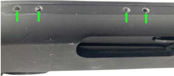
Begin by removing the (4) existing set screws from the top of the receiver using a flat head screwdriver as seen in (Figure 1a)
