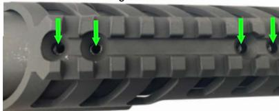
Next, slide the side saddle onto the receiver as seen in (Figure 1b), making sure the holes in the top of the receiver line up with the holes in the top of the side saddle as seen in (Figure 1c).
